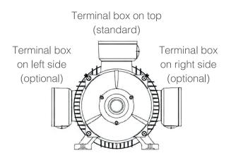
The terminal box position of OMPM series motor is on the top of house, drive end (standard position). It can also be located on right or left side of the house.
