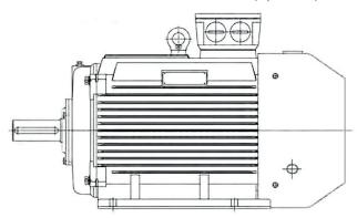
The terminal box can be rotated by 90°, so it is easy to adjust the cable entry to left right, drive end or non-drive end.
